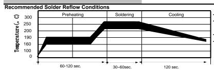
Recommended reflow methods : IR, vapor phase oven, hot air oven.
